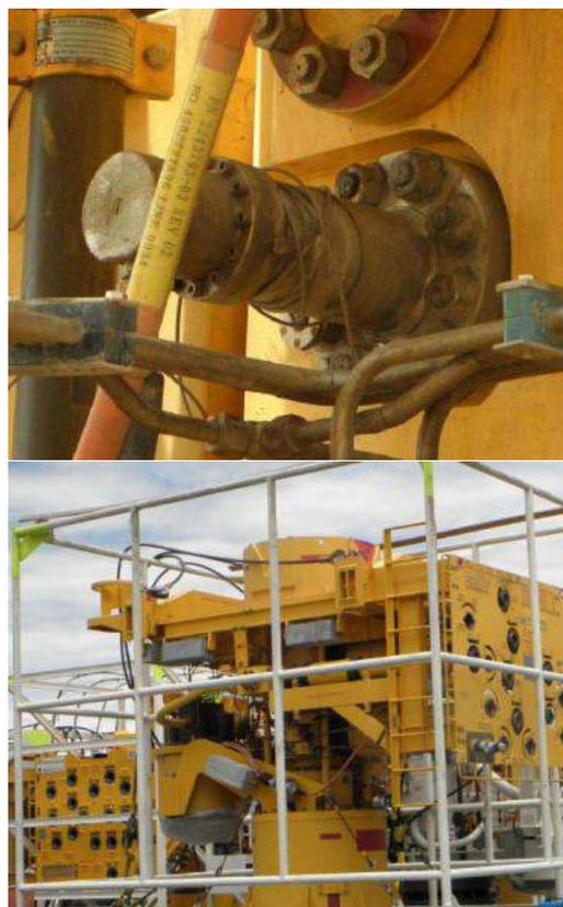
Fig. 1 Sensor installation at the X-mas tree for oil well monitoring.
