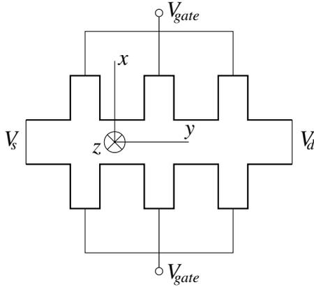
Fig. 1. Device geometry for the multiple-gate quantum stub transistor.  $V_s$  is the source voltage,  $V_d$  is the drain voltage, and  $V_{gate}$  is the gate voltage.
