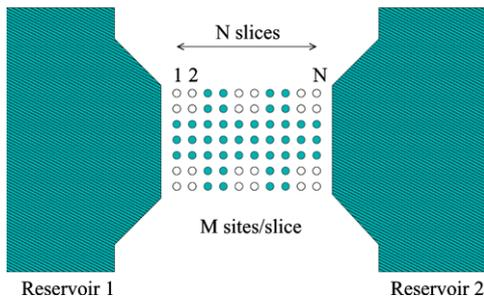
Fig. 3. Quantum device connecting two reservoirs. The device is divided in  $N$  slices, with  $M$  sites each, for a total of  $N \times M$  sites.
