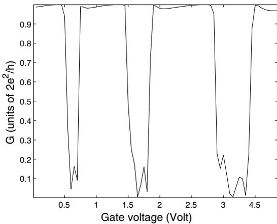
Fig. 6. In the triple gate configuration the block region is much wider. The voltage barrier is  $2E_F$ ,  $W = 10$  nm,  $a = 0.5$  nm, and  $L = 275$  nm (length of main wire). Stub length is 48 nm, and spaced 10 nm.
