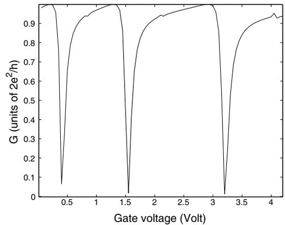
Fig. 4. Simulation of the quantum transistor with one pair of symmetrical stubs. The voltage barrier is  $2E_F$ ,  $W = 10$  nm,  $a = 0.5$  nm, and  $L = 275$  nm (length of main wire). Stub length is 48 nm.
