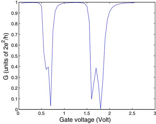
Fig. 5. Simulation of a double gate quantum stub transistor. The presence of the double gate generate a doublet. The voltage barrier is  $2E_F$ ,  $W = 10$  nm,  $a = 0.5$  nm, and  $L = 275$  nm (length of main wire). Stub length is 48 nm, and spaced 10 nm.
