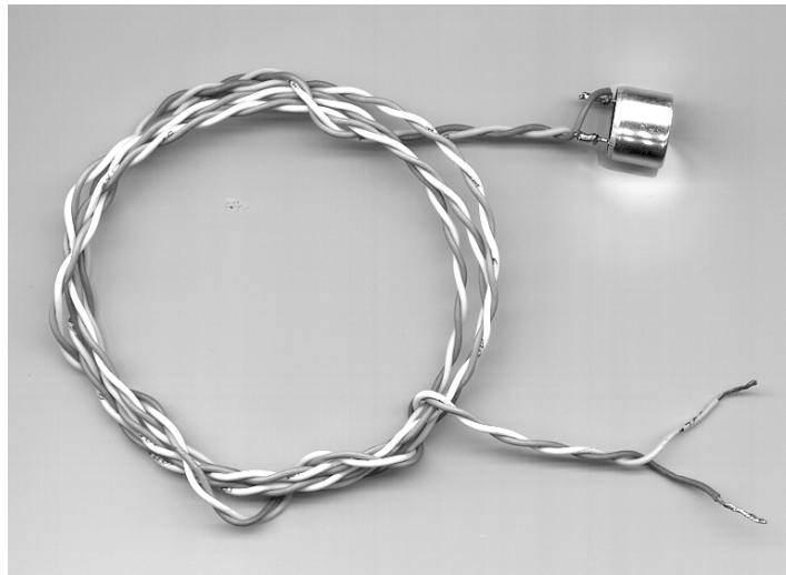
Ultrasonic transducer attached to wire leads.
