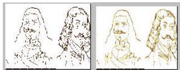
Fig. 5 - Reconstruction of a hand-drawn draft using 2D- legd2 . (a) Original (b) Reconstructed image from 1-level wavelet decomposition.
